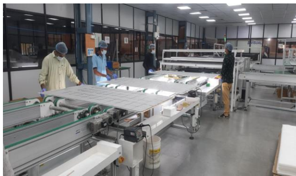
STRING TAPPING, SOLDERING AND CUTTING
