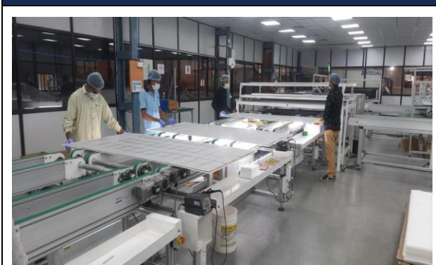
STRING TAPPING, SOLDERING AND CUTTING
