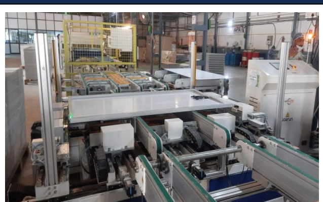
JUNCTION BOX INSTALLATION
