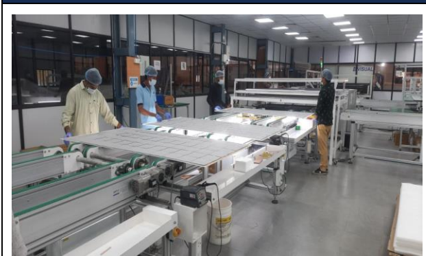
STRING TAPPING, SOLDERING AND CUTTING
